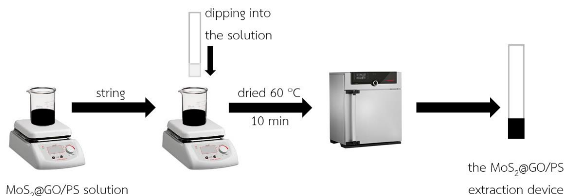
Figure 2: Schematic presentation of preparation of the MoS 2 @GO/PS composite coated on etched glass slide.
